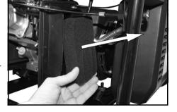
dry completely. Once it is dry, immerse in clean engine oil and squeeze to remove excess oil.
