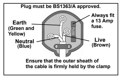
connected to the terminal which is marked E or  $\downarrow$  or coloured green.
