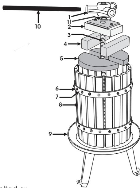
The base of the unit should be bolted or screwed to a firm, solid base, using the holes in the feet. (bolts not supplied)
