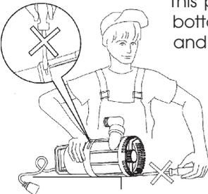
To replace the cover, ensure the notch in its periphery engages with the extended lug on one of the clip attachments on the base of the pump, (as shown in the diagram opposite), and press the cover home.
